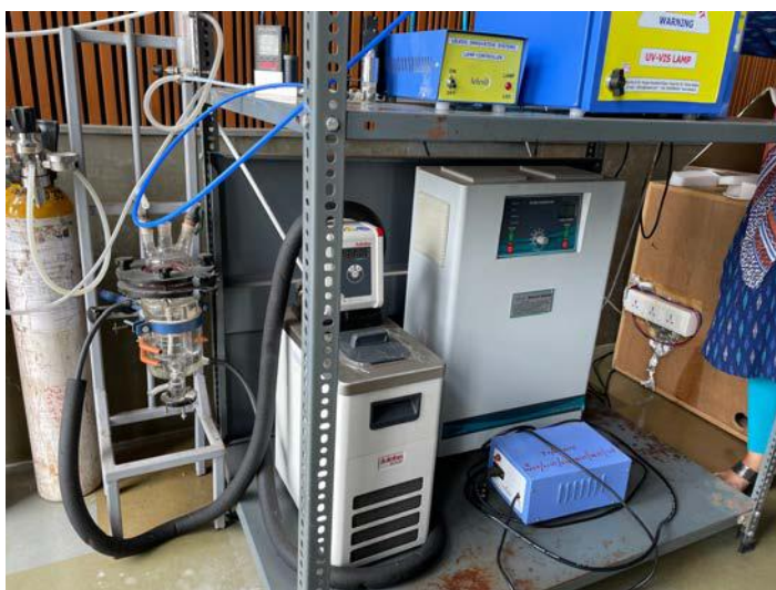
The ozonation set-up for Water and Flue gas treatment.
