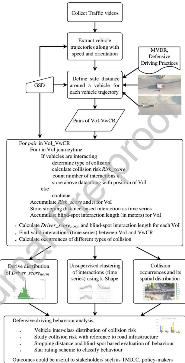
Figure A.21: Flowchart of defensive driving behaviour analysis methodology based on safe distance between vehicles.
