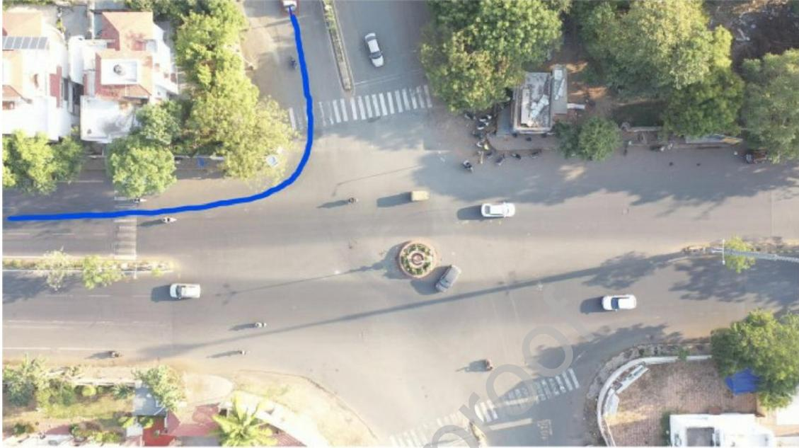
Figure 1: An example of vehicle detection and tracking. Refer to the track shown by the blue line.
