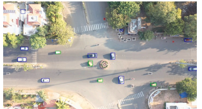
Fig. 5. An example frame showing bounding boxes for the vehicles detected using YOLOv7.
