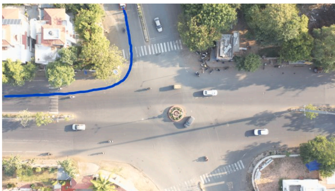
Fig. 6. An example of vehicle tracking using SORT.
